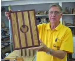
19mm Jarrah for contrast and strength. I thickened the board to 22mm and inserted a 80mm decal made with the oak and jarrah which
