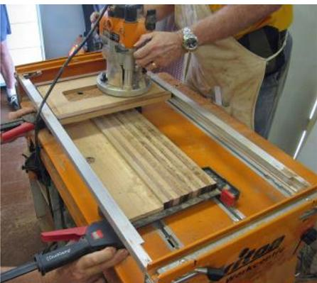
To mill wider boards, the board is moved on the table top. The board needs to be held firmly on the table top while milling work is done. The photo shows the jig ready for milling a cutting board."
