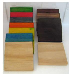
The photo at left shows a series of stains on identical samples of Radiata Pine. In the left row from the front is a piece of unstained Pine followed by the UBeaut Water Based that are food and toy safe of blue, yellow, orange, green/black, red, green. At right the front piece in unstained behind is Feast Watson Mahogany followed by Wattyl Teak then Feast Watson Red Cedar
