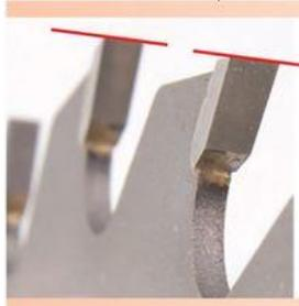
**Flat Top Grind (FTG)** teeth plow through the wood. They're primarily used on rip blades, where a fast feed rate is important to prevent overheating and bottom-side tear-out isn't an issue because the cut runs parallel to the wood fibers.
