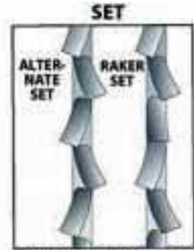
Alternate-set blades spread the work to ease cutting thick stock. Raker teeth cut cleaner by clearing chips better.
