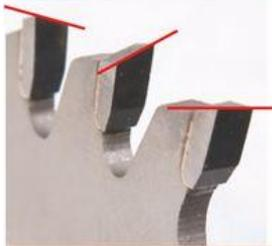
**Alternate Top Bevel/Raker (ATB/R)** This configuration groups crosscutting teeth and ripping teeth in five-tooth clusters. Designed for both ripping and cross-cutting, it's featured on 50-tooth combination blades.
