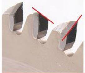
**High-Angle Alternate Top Bevel (Hi-ATB)** teeth have steep bevel angles (30 to 40 degrees) to cut melamine perfectly without tearing out the paper-thin face veneers. This tooth configuration is also great for hardwood plywood. These steeply beveled teeth are less durable than regular ATB teeth, though.
