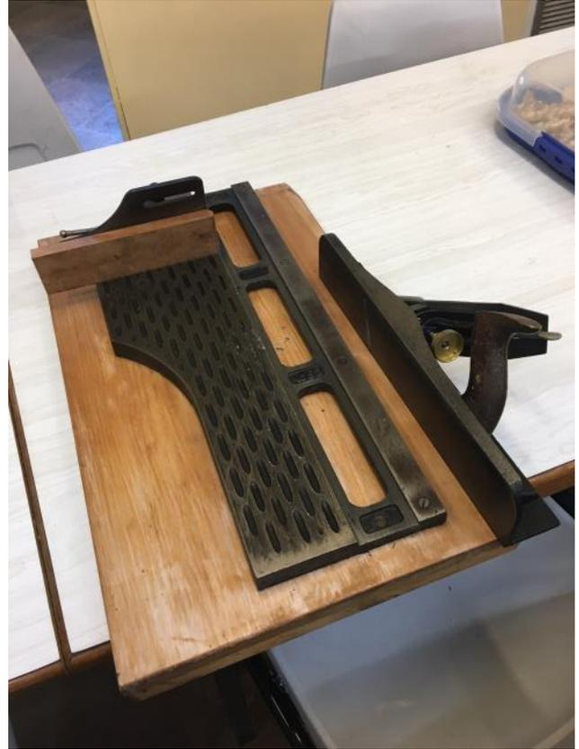
Above is a Stanley Shooting Board No 52 made between 1905 to 1943. Jim advised the Shooting Board is 22" long and 9" wide and weighs 35lb. with the Shooting Plane a Stanley No 51 made between 1909 and 1943. It is 15" long 2 3/8" wide and weighs 7 1/8lbs.
