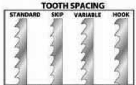
Standard blades cut aggressively, while skip-tooth blades clear chips to make smooth cuts. Variable-tooth spacing compromises on both. Hook teeth prove most aggressive, but dull faster.
