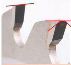
**Triple-Chip Grind (TCG)** teeth have beveled corners. On the blade, they alternate with FTG teeth. TCG teeth don't have scoring bevels, so they're very durable. They're used on glue-line rip blades and blades for melamine board, laminates and other manufactured materials when tooth durability is most important.
