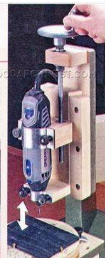
▲ Z Direction. The handwheel determines the depth of cut. Stick with shallow passes for cleaner cuts.
