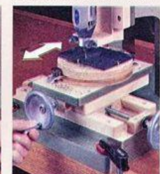
▲ Y Direction. Rotating the handwheel clockwise moves the workpiece toward the back of the machine.
