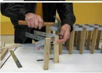
30mm square & 230mm long. I then cut a 'V' slot with the router into some scrap timber, clamped this to the band saw to guide the 30mm timber being cut I set up a stop and cross-cut each end diagonally. The metal strips were cut to 20 x 610mm and 14 x 890mm lengths and banged into the timber to construct the wine rack."
