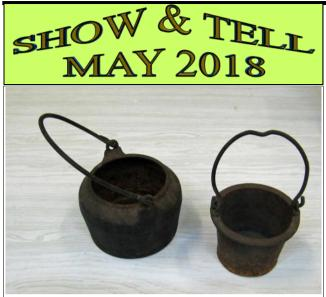
Ray T presented this Glue Pot and advised "The Glue Pot was my Grandfathers. When it came to our place Dad and I used it a lot until the late 1950's when PVA glue became popular. The Hide Glue pellets are melted to approximately 60-65°C and is useful for quick glue ups. Just coat, hold joint together until cool, and set aside to cure.
