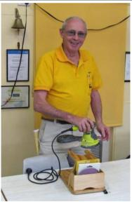
Ray presented this Random Orbital Stand and advised "While using my sander I got tired of waiting for the machine to stop before putting it down on the bench with parts still moving. With this stand you switch to sander off and hang it to let it stop without dancing around the bench."
