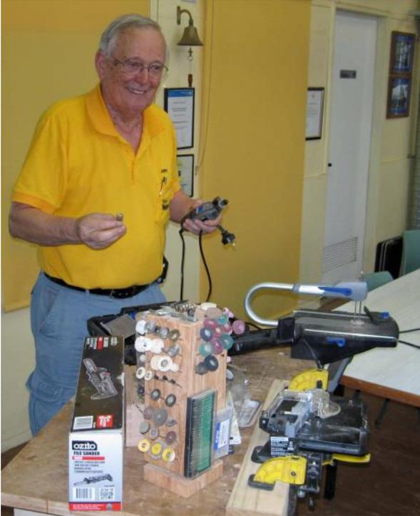
Please remember that the Dremel operates at speeds up to 33,000 RPM therefore before using it make sure you are wearing eye protection. The Dremel cuts, sands, shapes, drills, polishes, engraves, routes etc.
