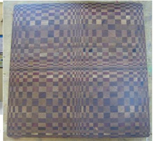
The process required a lot of cutting and sanding to precise measurements with thicknesses required ranged from 3mm to 24mm. Two boards were glued up with the second being a 'negative' of the first (ie; the order of the two timber types was reversed).
