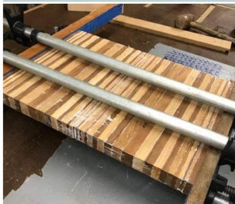
All the cutting gave me enough pieces for two boards and I'm now ready for the final glue-up on the second board. My thoughts on this one are to make it into a platter using a template and a bowl router bit to sculpt out various shapes within the board.
