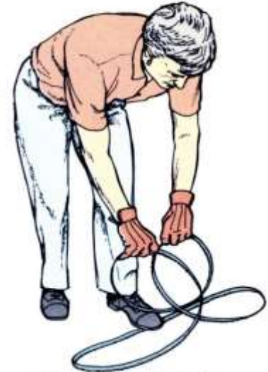
3 Cross the blade over to form three coils, then let it fall
