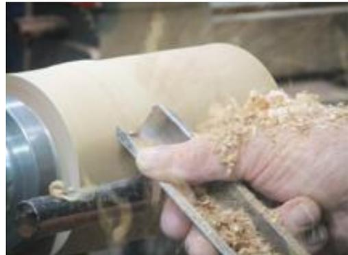
Law #4: The only part of the tool that should be in contact with the wood is that part of the tool that is receiving direct support from the tool rest.
