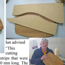
board was made from American Oak strips that were 40mm x 28 mm in section and about 450 mm long. The board used eight pieces and was glued and clamped together using Titebond waterproof glue.
