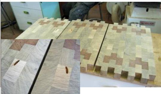
During the slicing process I encountered a worm hole that showed up on 2 surfaces. These were repaired by removing the top 10mm of each block with the hole and replacing timber from a spare block. After the final milling the repaired area was undetectable.
