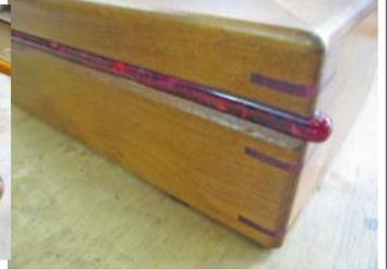
Ian also presented this Teak and Banksia Nuts box and advised "This box is made from some teak that was given to SWC in February. The box uses a different design hinge that is basically a 10 mm rod of acrylic that locates in 5 mm radius grooves cut into the base and lid.
