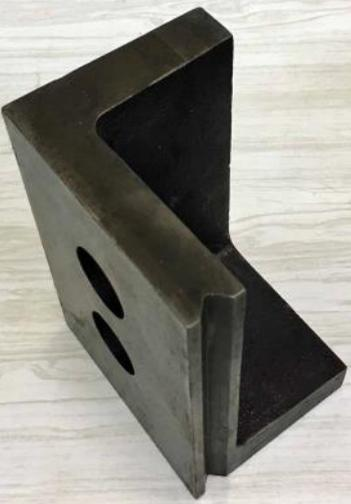
James Windschuttle our Club metalworker extraordinaire has provided the Club with this "hunk of steel" to enable us to quickly check that the fence on the jointer is at a perfect 90 degrees. It can also be used on any thing that a 90 degree angle is required. Many thanks Jim. The item is stored in the drawer below the Thicknesser.
