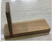
The drawer side to front useful when the drawer front extends beyond the side as would occur when there is a divider between and the drawer faces
