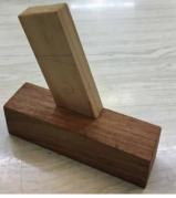
The other version is useful when jointing thicker to thinner wood and at an angle, or with curved to curved shaped
