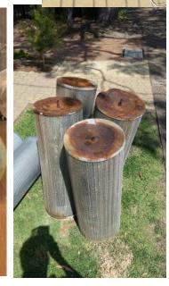
photos at right, have since been cleaned with compressed air gun with extended nozzle, washed out with pressure water, treated rust, painted where applicable, fitted new screwed rod, s/steel washers, nuts and lock nuts, packed in cardboard cartons and stored away for next service.
