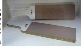
Over the years I have found that new Melamine Particle Board Sheeting -16 mm is a very stable and an ideal flat product for this project. If you intend using second-hand shelving material or timbers, check for distortion and/or twist before use. Whatever material you use, it is important to use a reliable straight edge to check that the surface is FLAT, also check the diagonals both ways for flatness.
