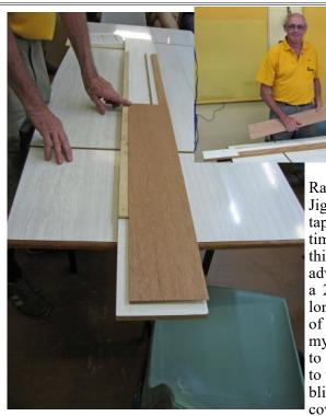
Ray presented this Jig to make a tapered splayed timber on the thicknesser and advised "I needed a 2400mm (2.4m) long splayed piece of timber to go on my weatherboard to plumb the wall to take a roll down blind with covering hood.
