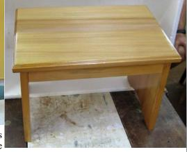
have been using a footstool at home that I made about 40 years ago & decided it needed replacement and a bit higher. I had a length of 300x35mm Queensland maple at home that would be suitable. Roger gave me some assistance with the band saw to reduce the thickness. This timber was good for the thicknesser, & Richard made good use of the offcut.
