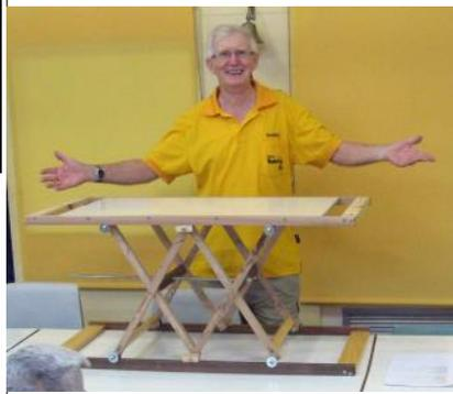
Maurice presented this scissor lift and advised "My scissor lift device. I was looking for a means of raising the height of a small, somewhat weighty, Ryobi bandsaw to use at a comfortable height instead of it being placed on my home workbench taking up too much bench space as well as being too high for comfortable use. I have a small workbench and
