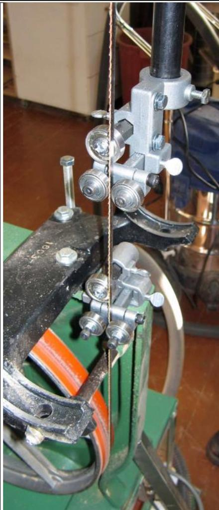
Our old 14" Hafco Bandsaw has had a bit of a facelift during this last month. The upper and lower blade guide bearing have been replaced as seen in the photo by a set of Baladonia Tools Bandsaw Blade Deluxe Guide Set.
