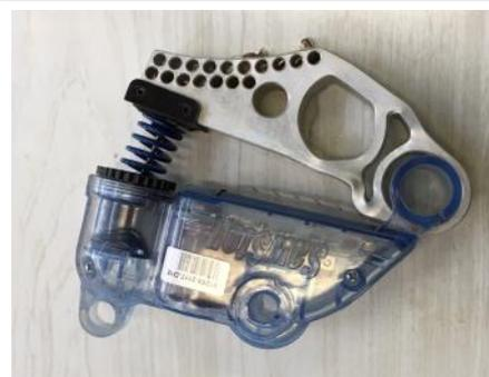
The photo at left is of a triggered cartridge from one of our Sawstop Table Saws. We have had to replace two of these in the last month. No, on either occasion did the triggered cartridge saved a finger or a hand.
