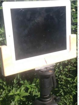
thicknesser and then sandwiched between two pieces of 7mm plywood. One piece of the plywood then routed to give a clear area for the iPad screen. The whole bracket comes up almost to the centre of the iPad, leaving the ntinued on page 8)
